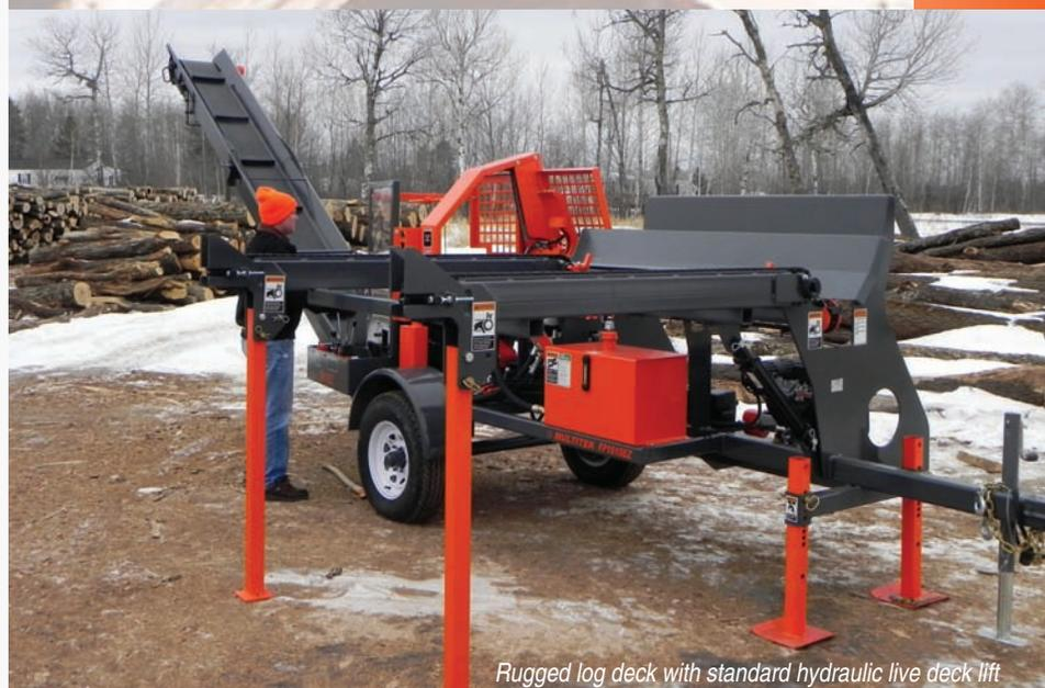
Rugged log deck with standard hydraulic live deck lift
