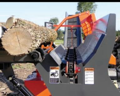
*Heavy duty log advance chain and engine guard*
