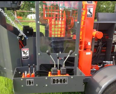
*Ergonomic operator safety station with 4-way Joysticks*
